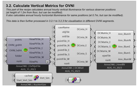
This subsection is the pre-cursor for its 4 sub-subsections, each of which evaluate various constituents of the OVNI diagrams. The annual illuminance for each occupant position (at horizontal plane at the table height for the OVNI hemisphere, and on vertical plane facing four orientations at the eye-height for the OVNI rings) are evaluated as CSV files in this sub section.
