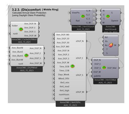
The calculations for visualization in OVNI middle ring: **Protection from discomfort glare** using evaluations of Daylight Glare Probability (DGP) for annual occupied hours – facing the four principal orientations, are performed by the following 6 components:
