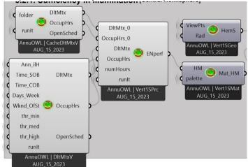
The calculations for visualization in OVNI hemisphere: **Daylight sufficiency performance** -- based on Daylight Autonomy compliance thresholds calculated for annual occupied hours, are performed by the 5 components in this sub-subsection.
