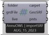
*pnts:* List of points for Radiance grid-based simulations Connections (Input): ExportSRF, PreCache, KeyCacheOBJ Connections (output): Custom Preview, GptFile
