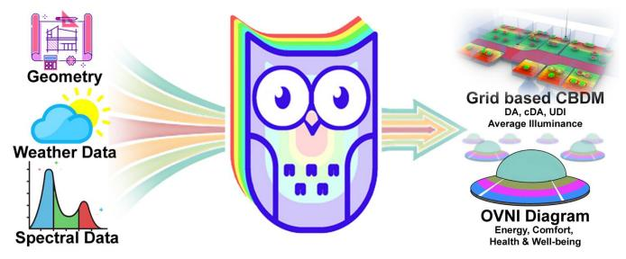
As user-input, AnnuOWL requires building geometry, weather data (as \*.epw file), and pre-calculated annual spectral data as (\*.aowl file). Other parameters, such as: occupancy schedule, table height, head height, grid
