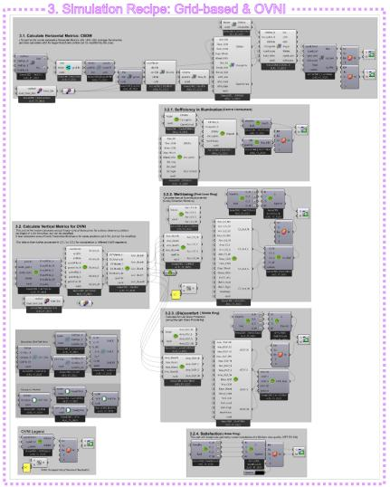
This is the pipeline with 43 components, nested under 3 subsections: for Horizontal grid-based evaluations, for OVNIbased evaluations, and supporting components. The components in this section form the main engine behind the AnnuOWL evaluations. The horizontal and vertical illuminance calculations are supported by Radiance 2-Phase Daylight Coefficient method for grid-based evaluations. This section does not need user-modifications.
