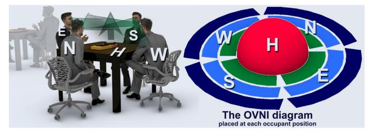
Each OVNI includes a hemisphere, surrounded by three rings. Each ring is sub-divided into four segments, facing North, East, South, and West orientations.
