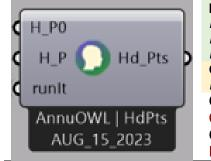
Inputs: H\_P0: (if pre-cached) Head positions of the occupants H\_P: (if live-sim) Head positions of the occupants runlt: A boolean toggle for this component. True = Live, False = Precache. Outputs: Hd\_Pts: Head positions of the occupants Connections (Input): CacheHPts, HPts, KeyVertSim Connections (output): DefVptFile
