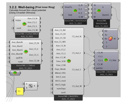
The calculations for visualization in OVNI first inner ring: **Circadian/Non-visual potential** using evaluation of Circadian Stimulus for annual occupied hours – facing the four principal orientations, are performed by following 6 components:
